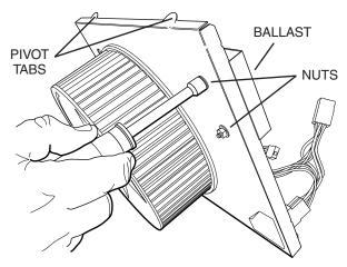
Remove (2) NUTS securing BALLAST using 11/32" socket or wrench. Remove ballast and dispose of appropriately, according to local laws and requirements
