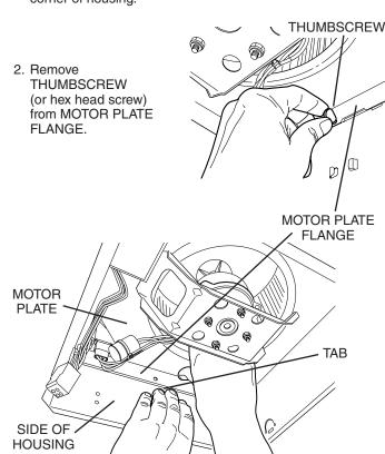
3. Find the single TAB on the MOTOR PLATE (located next to the motor's receptacle). Push up near motor plate tab while pushing out on SIDE OF HOUSING. Or insert a flat-blade screwdriver into slot in housing (next to tab) and twist screwdriver. Pivot motor plate down and remove.
