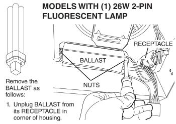
Remove (2) NUTS securing ballast using 3/8" socket or wrench. Remove ballast and dispose of appropriately, according to local laws and requirements. Continue to "INSTALL NEW GRILLE" section.
