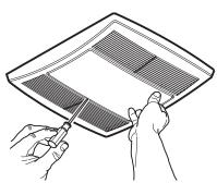
Remove light lens from grille by carefully inserting a small flat-blade screwdriver between grille and lens locking tab and prying lens out.
